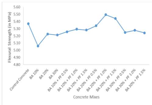
Fig. 4 Comparison of Flexural strength with various percentages of Bottom Ash & Polypropylene Fibre and Controlled concrete at 28 day's age of concrete.
