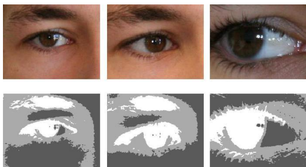
Figure 3 Examples of the results of K-Means Clustering on some images (a) Real Images (b) Clustering result images, white regions represent the estimated iris region
