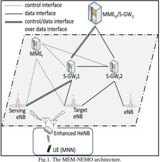
Under the LTE standard, a HeNB connects to the operators core network via a public network over a secure IP-based connection. configures the egress interface(s) of the enhanced HeNB to communicate with the MMEU and S-GWU via the IP connection in an LTE wireless access network. In other words, the enhanced HeNB's acts as a UE that connects to the serving eNB and is served by the MMEf and the S-GWf 1. Then forwarded from the MMEU/S-GWU to the enhanced HeNB via the S-GWf 1 and the serving eNB.
