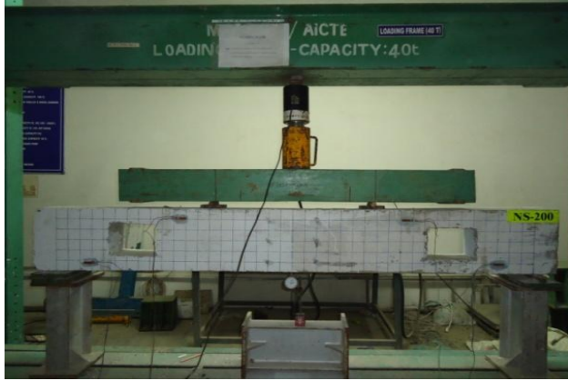
b) Beam with Duct Opening
