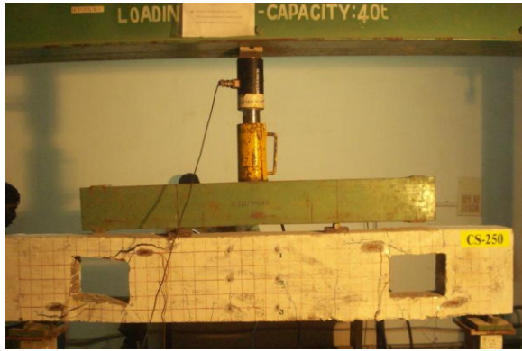
Fig. 10. The Deflected RC Beam with Opening
