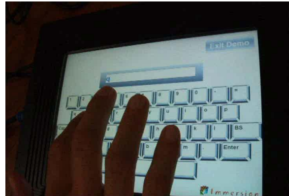
Figure 2: Immersion’s Touch Screen device for typing a keyboard with tactile sensations presented on an LCD display.
