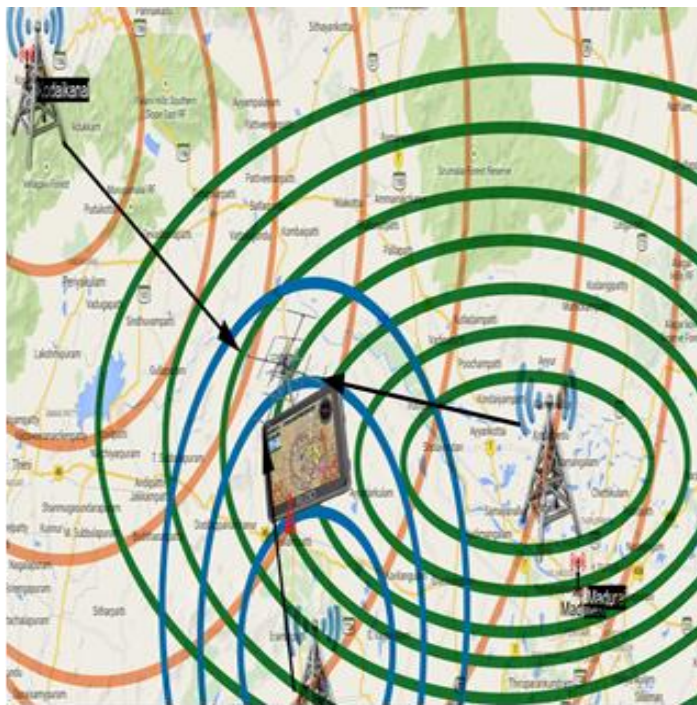
Fig. 6 Location using three towers
