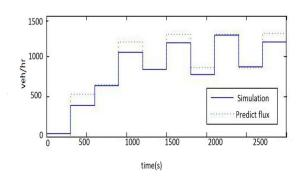
The above figure shows the vehicle discharge rate as number of vehicles per hour and time in seconds. As the time increases the predict flux differs from simulation result. This states that the algorithm used for prediction of traffic flow gives good result for short period of time.
