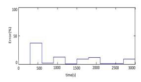
The above figure shows percentage error in simulation result and predict flux. Error in prediction increases as the time increases but gives nearly accurate result in case of short period of time.
