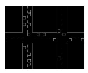
There are source nodes from which vehicles can enter into the network. There are six source nodes in a network element as given in the figure. There are crosses in the network where vehicles decide whether to take left turn, right turn or go straight. This model consists of double lane traffic. This is shown using simulation in c-language graphics.
