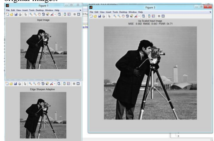
Fig 4.1 Input and Upscaled Image with Edge sharpen filter.
