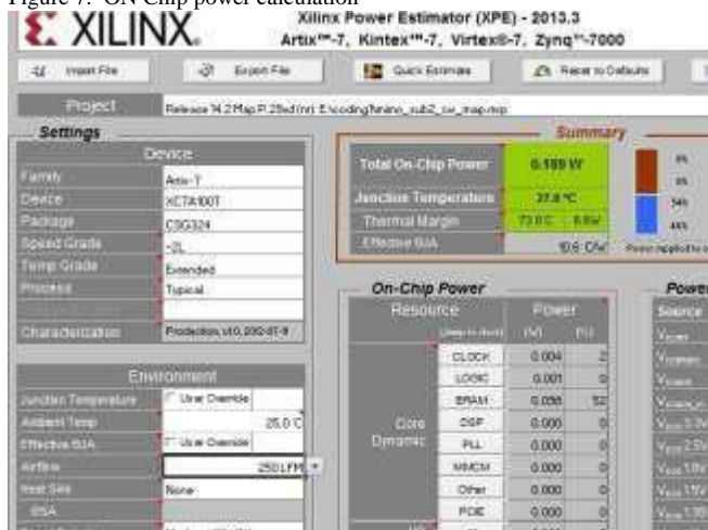
Figure 7. ON Chip power calculation
