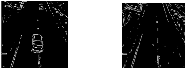
Figure 3(a) Figure 3(b) Figure 3(a), Edge detected foreground image Figure 3(b), Edge detected background image
