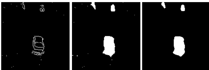
Figure 4 Figure 5 Figure 6 Figure 4, Image containing only vehicles on the road (subtraction module). Figure 5, Morphologically closed image. Figure 6, Binary image.
