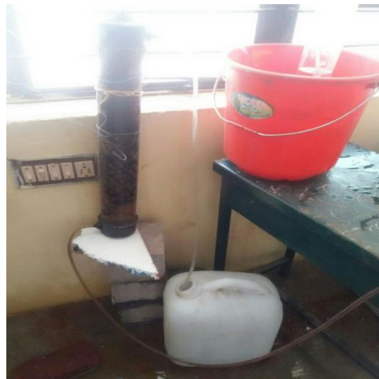
Fig. 2.4 Reactor Setup with Biogas Recovery
