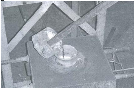
Figure 2: Pouring of Al-SiC melt into mold.
