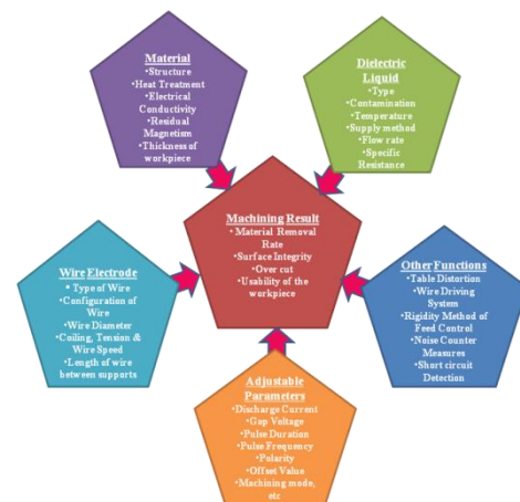
Figure 1 Factors Influencing the Wire EDM process [1]
