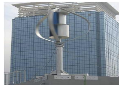
Figure 7. (a) 1.5kW VAWT [38]
