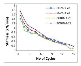
Figure 9. Stiffness Degradation curve of beam-column specimens on the 28th day
