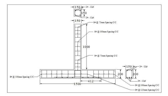
Figure 1. Reinforcement details of beam-column specimens
