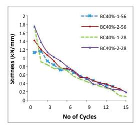
Figure 10. Stiffness Degradation curve of GGBS beam-column specimens
