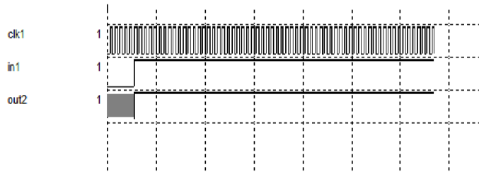
Figure 10: I/O waveform of Conventional D flip flop
