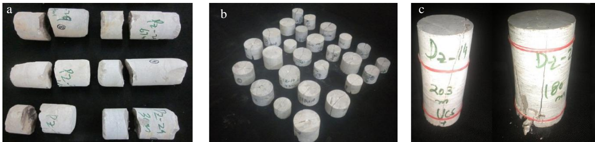
Figure 3 Failed samples after (a) PLT diametral (b) PLT axial (c) UCST
