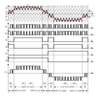
Figure 4 Switching logic of the proposed inverter.
