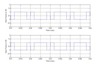
Fig 7 Switching pulses for S<sub>P</sub> and S<sub>N</sub> Switches.
