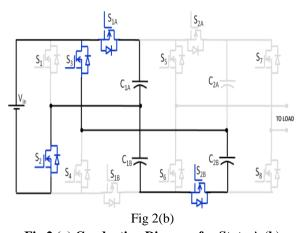
Fig 2 (a) Conduction Diagram for State A (b) Conduction Diagram for State B
