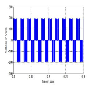
Fig 11 Load voltage with Modulation index = 0.5
