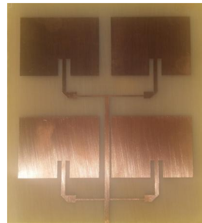
Fig. 10. Fabricated four Patch Antenna array
