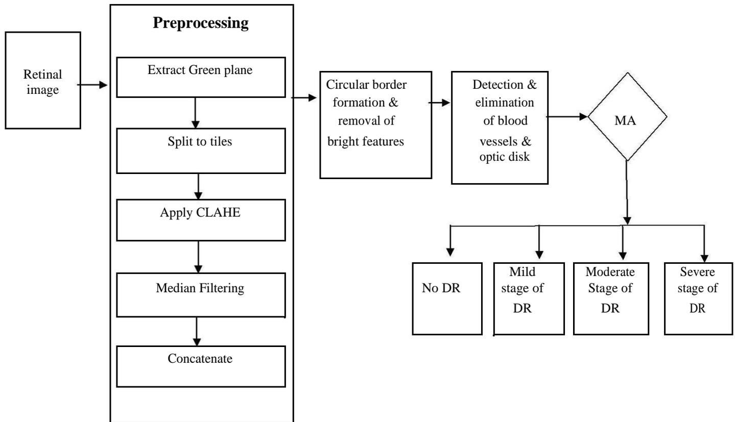
Figure 1. Block Diagram of the proposed system
