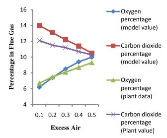
Figure 4.1 Variation of percentage in flue gases versus excess
