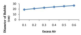
Figure 4.3 Variation of diameter of bubble versus excess air
