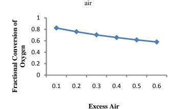
Figure 4.2 Variation of fractional conversion of oxygen versus excess air
