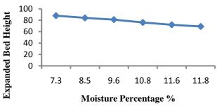
Figure 4.6 Variation of expanded bed height versus moisture percentage
