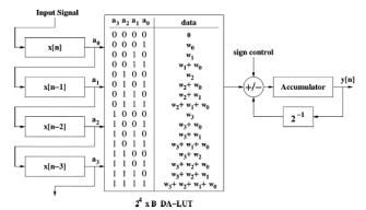
Fig.1. Block diagram of DA implementation of a 4-tap (k=4) FIR filter. Each coefficient has B bits of precision.
