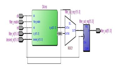
Fig 3. Top level circuit diagram of proposed DA adaptive filter.
