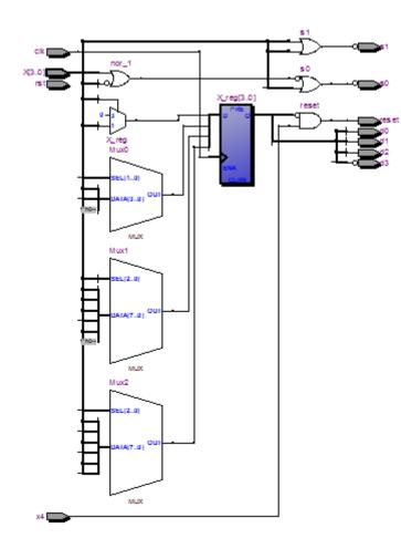
Fig.4. RTL schematic diagram of address generator and controller unit.
