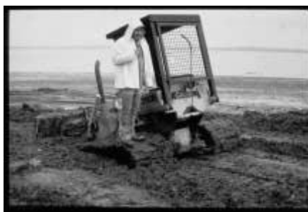
Fig. 1 Equipment mired in Muck
