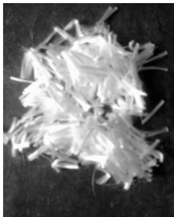
Fig. 3 Short Polypropylene(PP) Fibres
