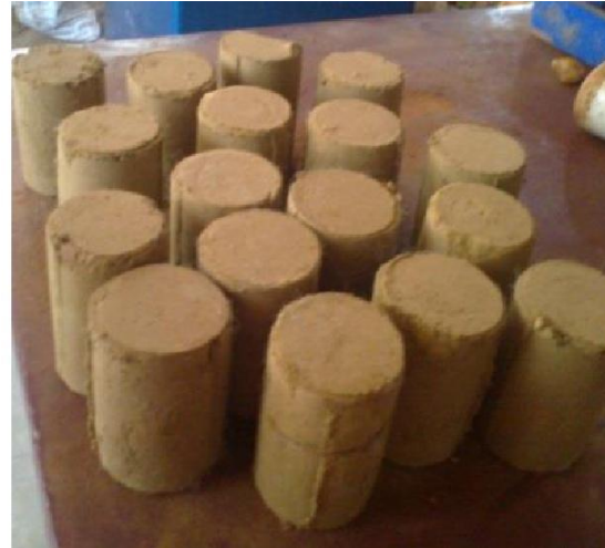
Fig. 6 Fibre reinforced soil specimen
