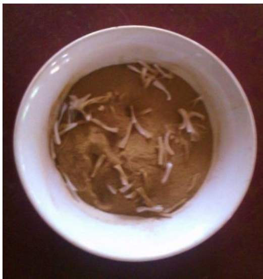
Fig. 5 Soil Specimen Randomly Mixed with Fibers
