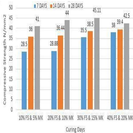
There is a considerable improvement in the compressive strength of concrete with inclusion and increase in the percentage of waste foundry sand up to 40%. It is observed that the compressive strength increased with increasing age of curing. The maximum compressive strength was achieved by 40% replacement fine aggregate with foundry sand.
