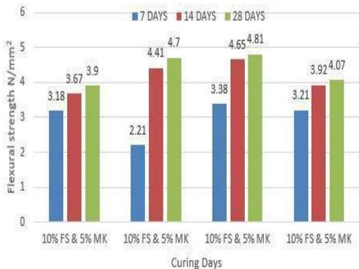
Increase in strength of various concrete mixtures over the plain concrete is also tabulated in the table 5. There is considerable increase in the flexural strength of concrete with the inclusion of foundry sand.
