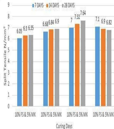
There is a considerable improvement in the split tensile strength of concrete with inclusion and increase the percentage of waste foundry sand up to 40%. It is observed that the split tensile strength increased with
