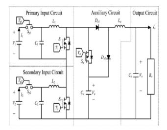
Figure 1. Equivalent circuit of high efficiency dual input converter
