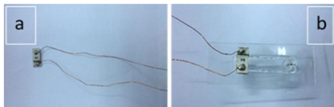
Figure 4. (a) The piezoelectric transducer of dimension: 1 cm x 1.2 cm. (b) Transducer placed and coupled in the back side of microfluidic device.
