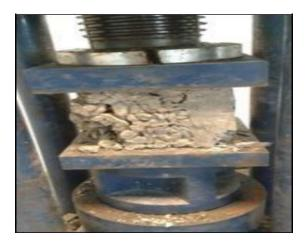
Fig 4.7 Compressive test on pervious concrete cube.
