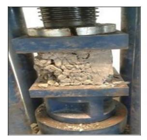
Fig-5.2 crack pattern of cube
