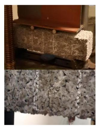
Fig 4.3 Loading and failure of pervious concrete beam without admixture
