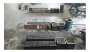
Fig 3.4 Beams and cubes after casting
