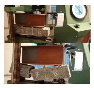
Fig 4.4 Loading and failure of pervious concrete beam with Conplast SP 337
