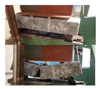
Fig 4.5 Loading and failure of pervious concrete beam with Conplast SP 430
