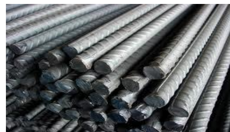
Fig.2 8mm dia Fe415 steel Bar
