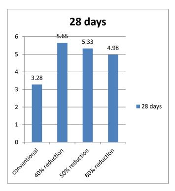
Summary: By comparing the result of split tensile strength of the cylinder with the ratio of 1:1:2, the greater strength is obtained in the mix with reduction of sand for about 40%.
