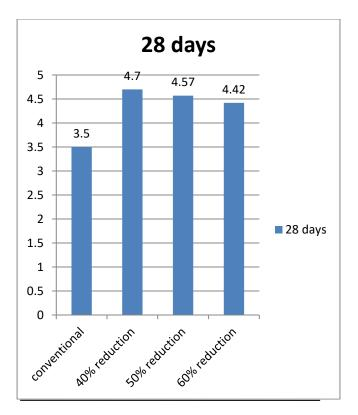
*Summary*: By comparing the result of flexural strength of the beam with the ratio of 1:1:2, the greater strength is obtained in the mix with reduction of sand for about 40%.
