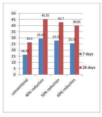
Summary: By comparing the result of compressive strength of the cube with the ratio of 1:1:2, the greater strength is obtained in the mix with reduction of sand for about 40%
