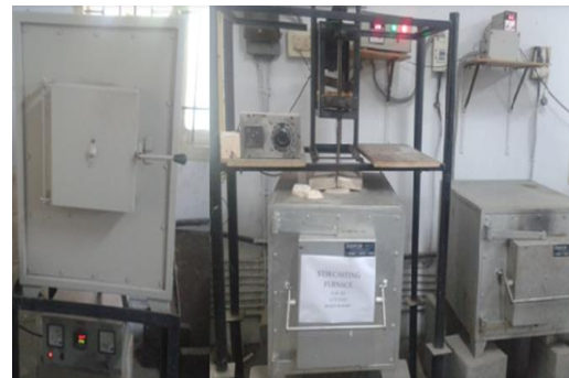
Fig 2: Stir Casting Set-up used for fabrication of Composite Plates (Al 7075/WC)
