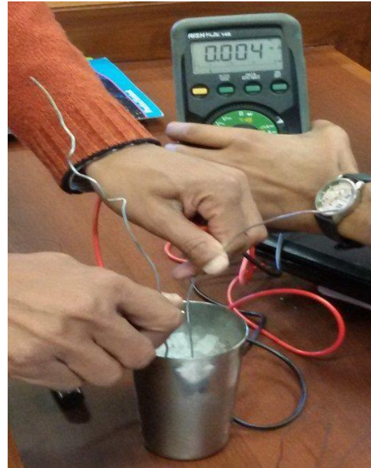
Figure 2 : Iron aluminum thermocouple with one junction in ice.
