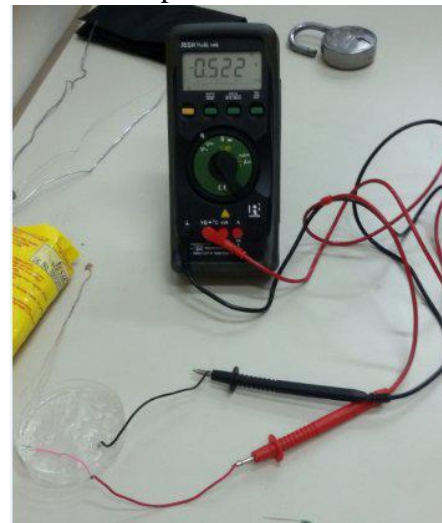
Figure 3 : Paper clip-Copper wire thermocouple in ice
