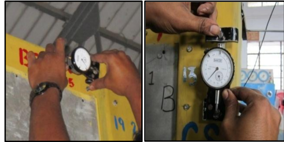
Fig.9 Measurement of strain in columns and beams
