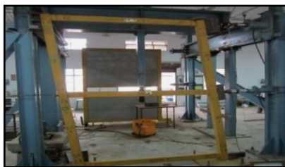
Fig.25 Deformation of Bare Frame–Frame (1)
