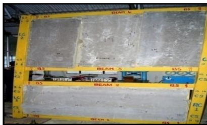
Fig.26 Failure Pattern of Frame (2)
