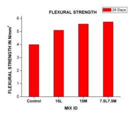
Fig.12 Test Results for Flexural Strength
