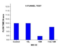
Fig.6 V Funnel Test Results
