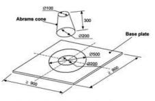
Fig.1 Slump Flow Test Apparatus
