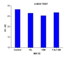
Fig.8 U Box Test Results
