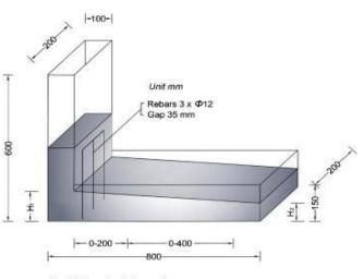
Fig.3 L Box Test Apparatus
