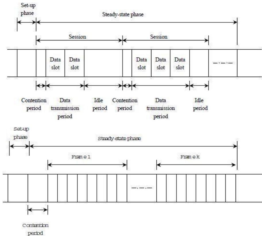
Fig. 1. The operations of BMA (top diagram) and TDMA (bottom diagram) are divided into rounds. The clusters are formed during the set-up phases. Each round ends after a predefined time and then the whole process is repeated.
