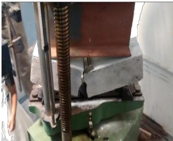
**Fig 4.2 Loading and failure of conventional concrete beam**
