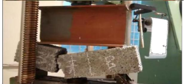
**Fig 4.4 Loading and failure of pervious concrete beam with Conplast SP 337**
