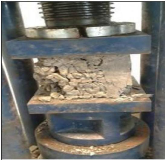
Fig-5.2 crack pattern of cube
