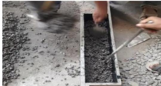
**Fig 3.3 Casting and tamping of concrete**
