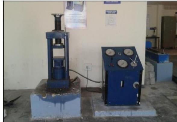
**Fig 4.6 Compressive strength Testing Machine (2000KN)**
