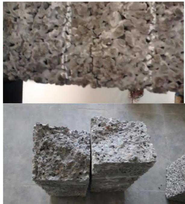
**Fig 5.1 Crack and failure pattern of beams**
