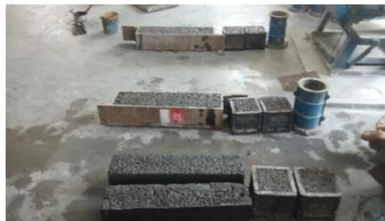
**Fig 3.4 Beams and cubes after casting**
