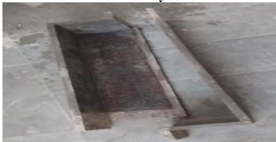
**Fig 3.2 Beam mould of size 700mm x 150mm x 150mm**
