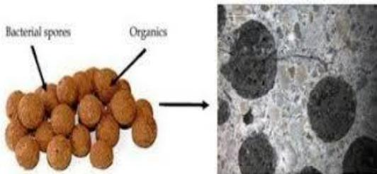
Fig: 1 Self healing admixture composed of expanded clay particles loaded with bacterial spores and organic bio mineral precursor compound (calcium lactate).when embedded in concrete matrix
