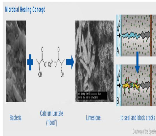
Fig 2. Microbial Healing process in concrete bacteria reacting with calcium lactate
