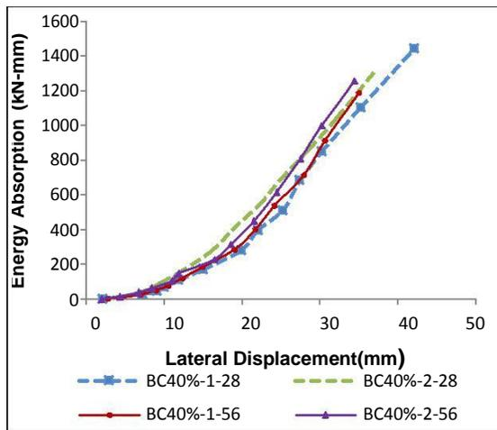
Figure 12. Energy absorption curves of GGBS beam-column specimens
