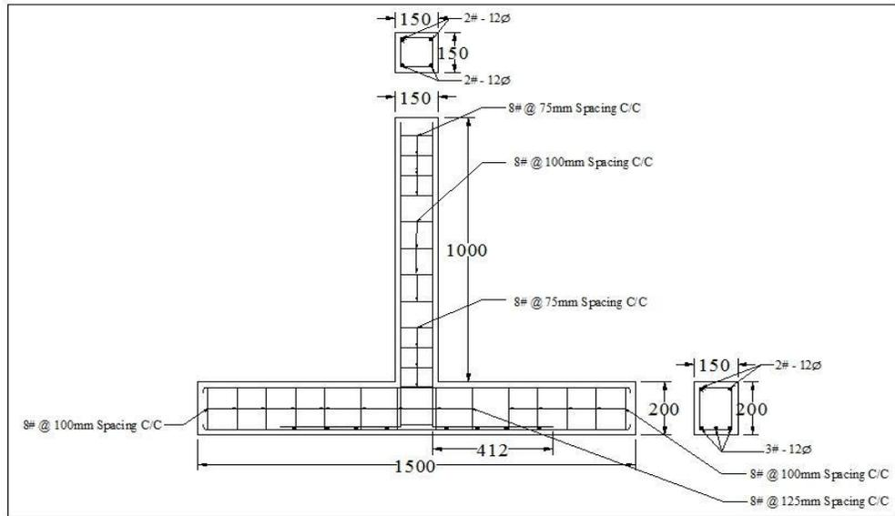
Figure 1. Reinforcement details of beam-column specimens
