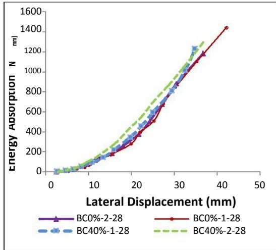
Figure 11. Energy absorption curves of the beam-column specimens on the 28th day
