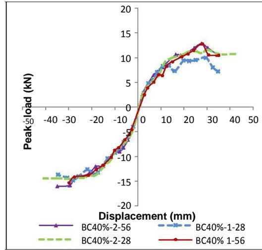
Figure 8. Peak load-displacement curves of the GGBS specimens
