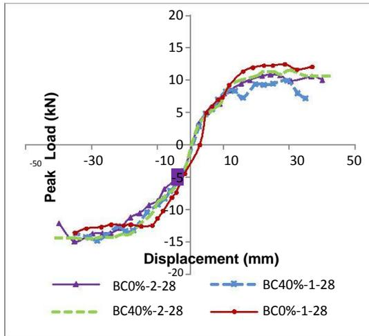
Figure 7. Peak load-displacement curves of specimens on the 28th day
