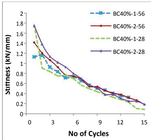
Figure 10. Stiffness Degradation curve of GGBS beam-column specimens
