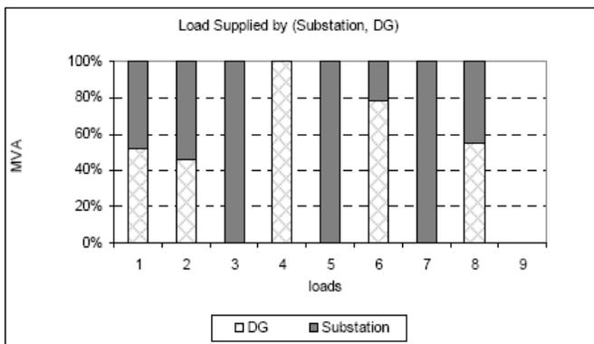
Figure 2.2 Load Supplied by Substation and DG for the DG option
