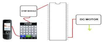
• The door security system consists of a DTMF module which is connected to a mobile phone permanently.
