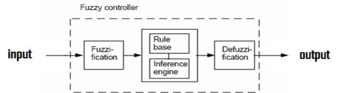
Figure 2. Structure of Fuzzy logic control
