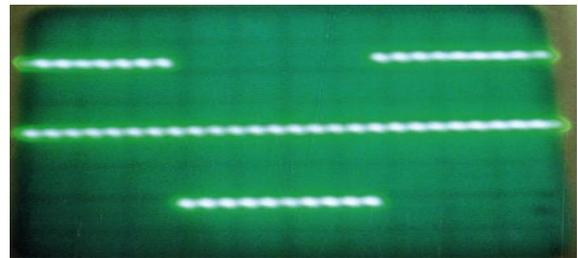
Fig. 4 (b). The output voltage of inverter with R-load
