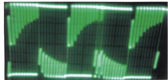
Fig. 4 (c). The output voltage of inverter with inductive load
