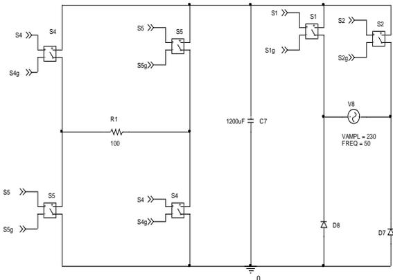
Fig. 2. AC to AC PWM converter with R load
