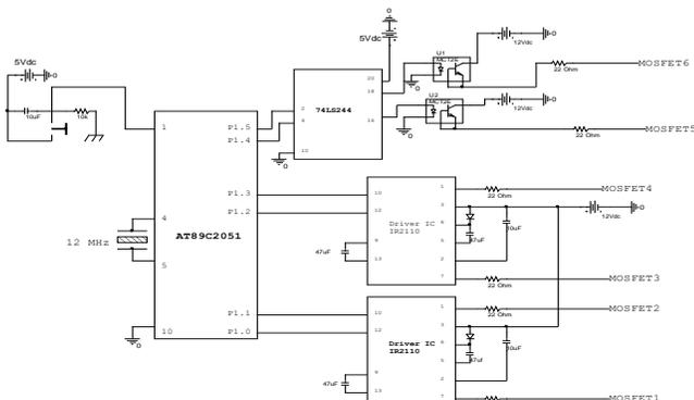
Fig. 4. Block Diagram of Control Circuit
