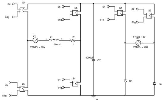
Fig. 3(a). AC to AC PWM converter with RLE load
