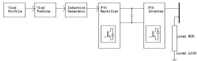
Fig . 1. Block diagram of variable speed induction generator system
