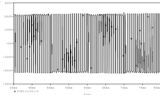
Fig. 3(b). Inverter Output for RLE Voltage
