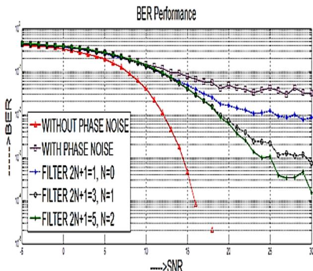
Figure.6. BER comparison with and compensated Phase noise (1)
