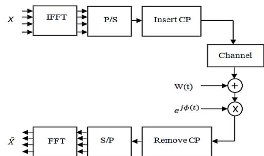
Figure.1. OFDM Transceiver
