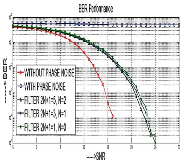
Figure.7. BER comparison with and compensated Phase noise (2)
