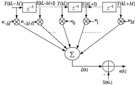
Figure.2. Phase Noise Compensation Filter
